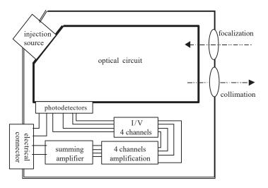
**Fig.5** : scheme of a measuring head
