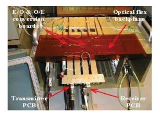
Fig. 9. Integrated optical backplane interconnect breadboard
