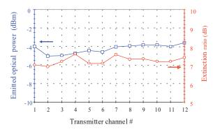
Fig. 2. Optical power and extinction ratio under 2.5 Gbit/s PRBS modulation vs. transmitter channel
