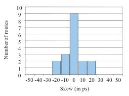
Fig. 8. Distribution of differential delays through the optical fibre routes
