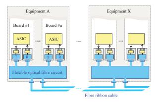
Fig. 1. Optical fibre interconnect for high-speed intraand inter-equipment communications
