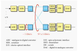
Fig. 7. An example of digital transparent processor architecture with optical interconnect (in blue)
