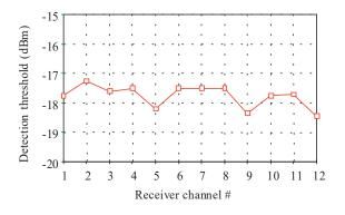
Fig. 4. Detection threshold at 10<sup>-9</sup> BER under 2.5 Gbit/s, 2<sup>7</sup>-1 PRBS modulation vs. receiver channel
