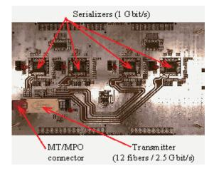
Fig. 6. O/E transmitter mezzanine board
