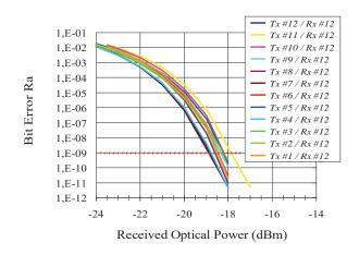
Fig. 3. BER performance under 2.5 Gbit/s, 2<sup>7</sup>-1 PRBS modulation vs. transmitter channel
