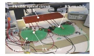
Fig. 7. Experimental set-up for testing the flexible optical fibre circuit
