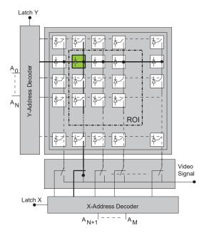
Figure 1 Typical APS detector matrix configuration
