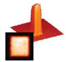
Figure 3 Spatial sensitivity distribution of a TFC pixel with near 100% fill factor
