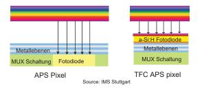
Figure 2 State of the art pixel cell technologies of APS detectors
