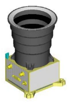
Figure 5 Geo-telecom APS star tracker configuration as a single box design solution
