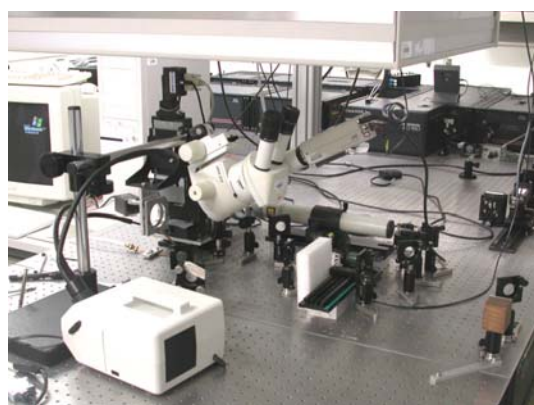
Fig. 4 Photograph of the laser damage setup with flowbox (above).
