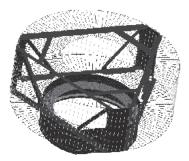
Figure 17: Internal stiffening structure between vane S1 and 1.
