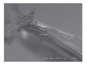
Figure 20: Painted then milled aluminium sheet
