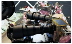
Fig.2: HRS telescopes during integration and alignment on the main structure
