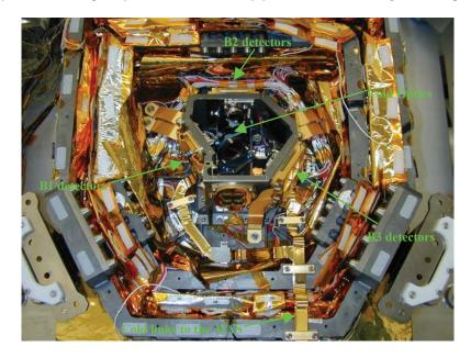
Fig. 1. Detectors integrated in Cold Box
