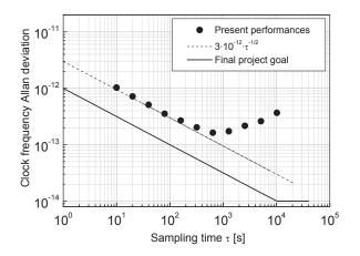
**Figure 2:** Typical stability performance of the modular Rb clock from Fig. 1 in terms of the Allan standard deviation.
