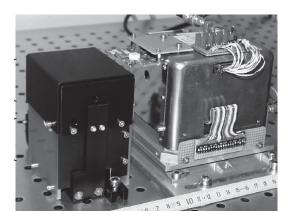
**Figure 1:** The modular laser-pumped Rb frequency standard. Left: Stabilized laser head module, including the reference cell. Right: lamp-removed Rb clock unit.
