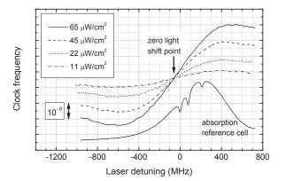
**Figure 5:** Light shift of the clock frequency as a function of pump light frequency and intensity. Frequency detuning is given relative to the cross-over resonance arising from the <sup>87</sup>Rb F=2 $\rightarrow$ 1 and F=2 $\rightarrow$ 3 transitions in the (laser) reference cell (denoted CO 21-23 in the text).
