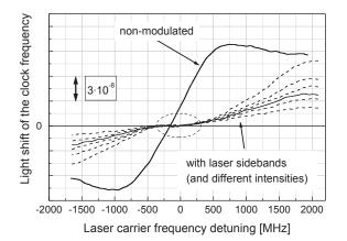
**Figure 6:** Light shift reduction by multifrequency optical pumping achieved by frequency modulation of the laser output. The dashed curves span incident pump light powers ranging from 36 to 105  $\mu$ W. Both solid curves refer to the same incident power of 55  $\mu$ W.
