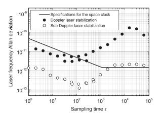
**Figure 3:** Laser frequency stability performance for stabilization to sub-Doppler saturated absorption or simple Doppler-broadened Rb vapor absorption lines. The stability specification is derived from the slope of the light shift curves in Fig. 5 for typical clock operation conditions.
