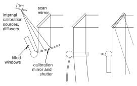
Figure 4-3 Deployment of separate components for absolute calibration and flat fielding
