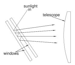
Figure 4-2 Ratioing concept with mirror and window
