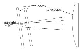
Figure 4-1 Ratioing method using windows
