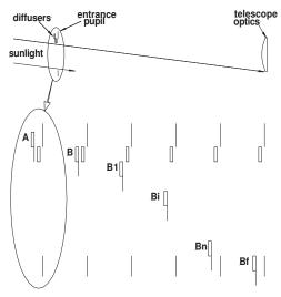
Figure 3-1 Ratioing method using 2 diffusers
