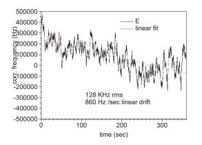
Fig. 4: First measurements of frequency stability of a RL locked to a cavity resonance.
