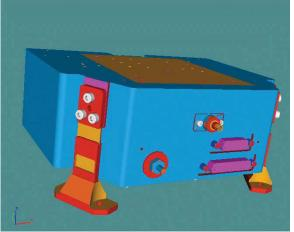
Fig. 6: RLH housing, showing isostatic mounts and connector interface.
