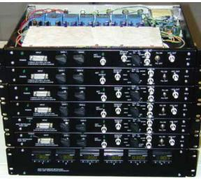
Fig 11. Photo of JWST/TPF metrology post-amps. Top module is open, showing multiple power supplies (rear) and the constant temperature oven (front). The bottom module is a six-channel temperature controller maintaining the ovens at 30.0 C.
