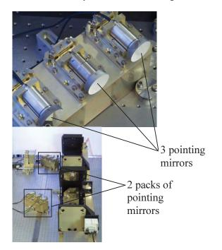
Fig. 3. On the top part is the first pack of 3 pointing mirrors. The central one is not actuated by piezo. On the bottom part are shown the 2 packs determining the homothetic mapping. The piezo actuators allow tip/tilt and piston (required for accurate OPD control) adjustments.
