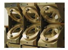
Fig. 5. These are the three delay-lines. A pair of flat mirrors composes each delay-line. The disposition is forming a right angle. The light is coming into the top mirror, is reflected onto the second mirror and then is leaving the delay line on the same vertical plan as it was coming. The left delay-line and the right one are actuated by piezo.
