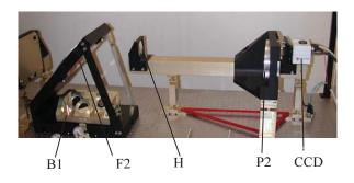
Fig. 4. The beam combiner is composed by the flat mirror on the left F2, the block of 3 fixed mirrors below it B2, the parabolic mirror on the right P2, the hyperbolic mirror in the center H and the CCD camera on the right.
