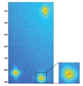
Fig. 7. Three stars observed within DTI with fringes on them simultaneously. On the right hand part it is shown that the fringes, are almost centered on the envelope.
