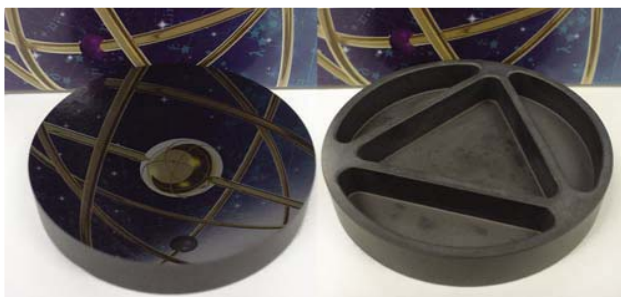
Fig. 5 Finished φ80mm sintered SiC mirror by ELID grinding
