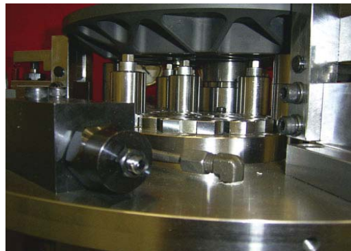
Fig. 12 The state where supports are in contact with \phi 360 mm sintered SiC mirror
