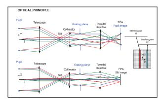
Fig.1 Optical concepts of heterodyne imaging spectrometer
