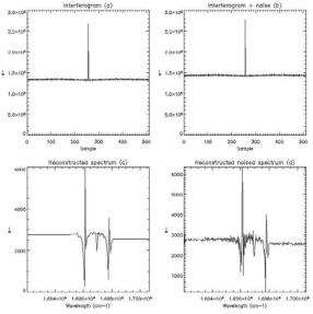
Fig.3 Initial spectrum (c) and its interferogram (a). Reconstructed spectrum (d) and its interferogram (b).
