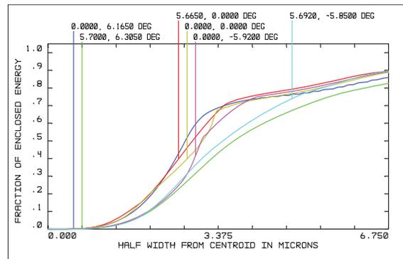
Fig. 3 Ensquared energy scaled by diffraction limit at a wavelength of 640 nm.
