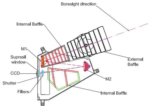
Fig. 4 WAC opto-mechanical design scheme.
