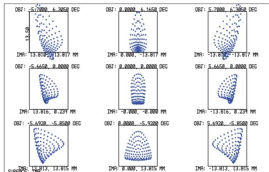
Fig. 2 WAC spot diagrams for the center, the edges and corners of the CCD. The overlapped boxes correspond to the actual pixel size of the detector (13.5 μm).
