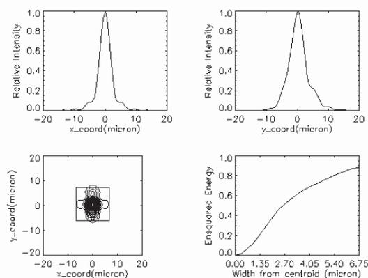
Fig. 8 Theoretical performance at the center of the FoV: PSF cross sections, spot diagram and EE.
