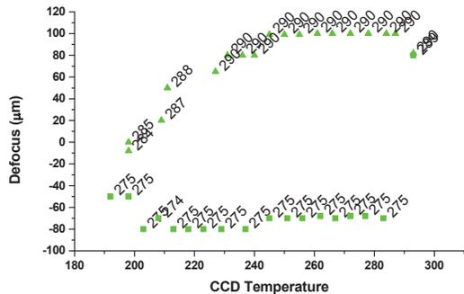
Fig. 10 WAC defocus versus CCD and structure temperature. The temperature of the structure is shown as label to the measurement points.
