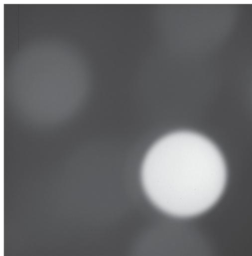
Fig. 15 Flat field image acquired illuminating the camera with the integrating sphere using the halogen lamps. The used filter is one with UV bandpass.
