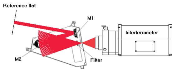
Fig. 7 Interferometric setup for alignment checking.
