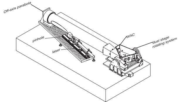
Fig. 5 Schematic of the laboratory facility used for testing the in-air WAC optical performance.
