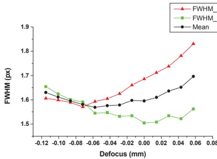
Fig. 13 Through focus measurements keeping cold both CCD and structure.
