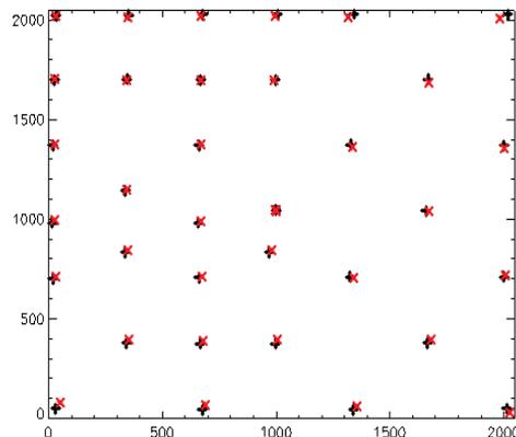
Fig. 14 Theoretical distortion (+) versus measured one (x). The difference between the two has been multiplied by a factor 20 to be visible.
