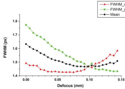
Fig. 11 Through focus measurements at ambient temperature. FWHM in x and y direction and mean values are plotted.
