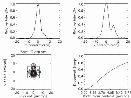
Fig. 9 FM measured optical performance at the center of the FoV: PSF cross sections, spot diagram and EE.
