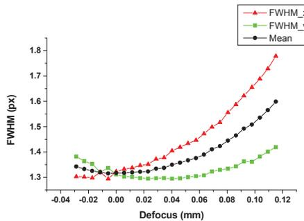
Fig. 12 Through focus measurements for CCD and structure at nominal operating temperature.
