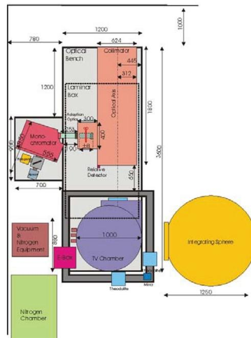
Fig. 6 Schematic of the laboratory facility used for testing the in-vacuum WAC optical performance.
