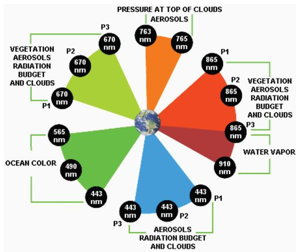
Fig. 3. Spectral and polarization channels with mission purposes.
