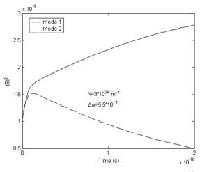
Fig. 2. Field intensities versus time for  $\Delta \omega = 5.5 \cdot 10^{-12}$
