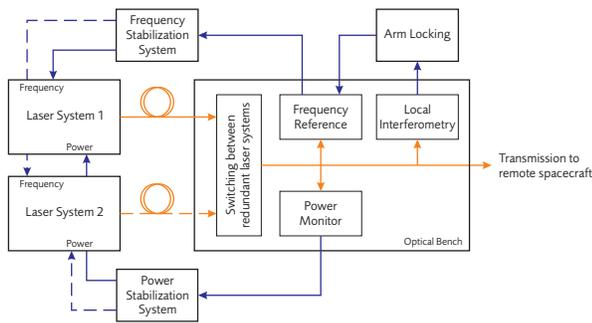
Figure 2. Frequency and power stabilization scheme.
