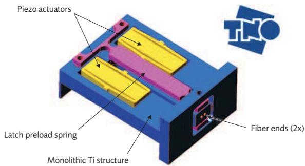
Figure 4. Conceptual design of a bistable fiber redundancy switch for integration on the LISA optical benches.
