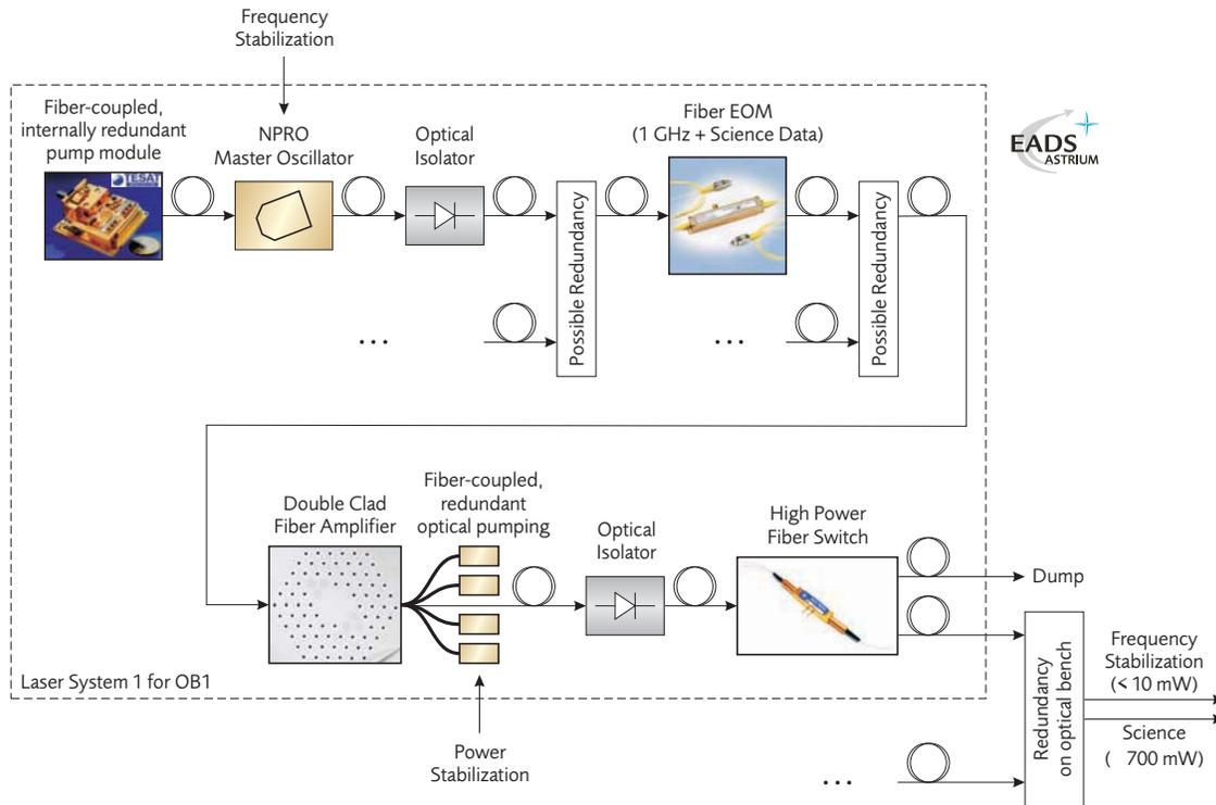
Figure 1. Overview of a possible MOFPA laser system for LISA. For concreteness, the schematic assumes the use of a low power diode pump module by TESAT for the master oscillator, a  $\text{LiNbO}_3$  broadband waveguide EOM by Guided Color Technologies GmbH, and a NanoSpeed High Power  $1 \times 2$  Solid-State Fiberoptic PM Switch by Agiltron.
