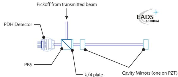
Figure 3. Typical setup for frequency stabilization to a cavity reference. The setup would be installed together with all interferometers on the optical bench. It would thus profit from the high dimensional stability provided by the Zerodur baseplate and the exceptional temperature stability of  $10^{-5} \text{ K}/\sqrt{\text{Hz}}$ .
