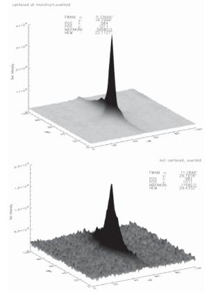
Fig. 2-4: Results of tests with a 3keV, 100μm pencil beam Overlaid spots reflected through 46μm square pore multifibre; 1px = 1.77". Spots centred on their maxima (top, HEW 22") and raw images overlaid (bottom, HEW 29")
