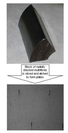
**Fig. 2-2:** Fused block of radially stacked micro-pore material above. Microscope image of sliced & etched plate below, one MF visible with surrounding MFs
