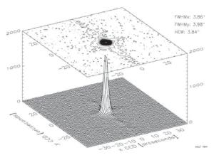
**Fig. 3-4:** First recorded reflection of an x-ray beam imaged by a silicon pore optic, integrated and fixed in Wolter-I configuration<sup>10</sup>.
