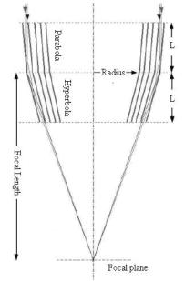
**Fig. 1-1:** Conical approximation of the parabolic and hyperbolic sections of a Wolter I optic to focus x-rays.
