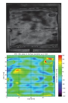
**Fig. 3-1:** Above, interferogram w.r.t. to a CGH, recorded at wavelength 633 nm, on the 2<sup>nd</sup> silicon plate that is stacked onto a Zeiss polished mandrel, which is larger than the plate and also visible. Central horizontal lines are artefacts caused by the CGH. Bottom image shows surface deviation of the
