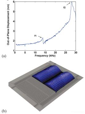
Fig. 6. (a) Doppler Interferometer measurement of the first and second resonant mode frequencies for the structure with periodicity of 9 µm. They are located at 13.8 kHz and 28.1 kHz, respectively. (b) Experimentally measured resonant mode of the structure when resonating at 28.1 kHz.
