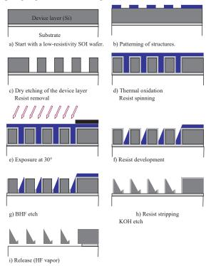
Fig. 9. Process flow for the blazed deformable MEMS gratings. This process adds steps (d) to (h) to the process for the planar deformable MEMS gratings (Fig. 3). Using KOH etch, an optically smooth surfaces can be obtained, corresponding to {1 1 1} Silicon planes. The entire process requires two masks.
