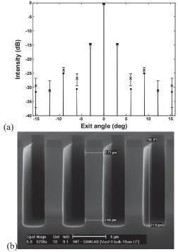
Fig. 7. (a) Intensity of diffracted orders for the 12  $\mu$ m period grating at normal incidence at the He-Ne laser wavelength of 632.8 nm. Good agreement is obtained between experiments and optical simulations using data derived from geometrical characterization. (b) Geometrical characterization of the 12  $\mu$ m period grating (SEM cross-section in a test wafer).
