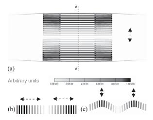
Fig. 2. (a) First (in-plane) resonant mode for the deformable MEMS grating with periodicity of 9  $\mu$ m. (b) Cross-section A-A' of the structure in Fig. 2(a) for the first (in-plane) resonant mode. (c) Cross-section A-A' of the structure in Fig. 2(a) for the second (out-of-plane) resonant mode.
