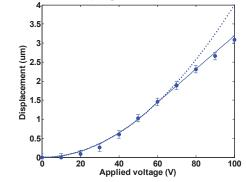
Fig. 5. Measured (dots) and simulated (solid line) displacement versus applied voltage for the 9  $\mu$ m period grating. Maximum displacement at each grating end is 3.1  $\mu$ m. Good agreement is obtained with simulated behavior. A deviation from ideal quadratic behavior (dotted line) is related to the design of the anchor points.
