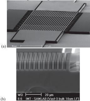
Fig. 4. Fabricated devices on a Si test wafer. (a) Top View of an entire device (optical microscope). (b) Cross-section SEM image of the spring region for one test structure with  $6 \mu m$  period.
