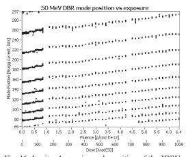
Fig. 16 In-situ change in mode position of the JDSU DBR laser exposed to 50 MeV protons.
