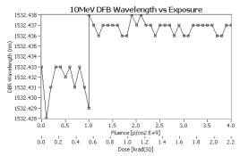
Fig. 6 In-situ wavelength measurement of Avanex DFB laser during irradiation with 10 MeV protons.
