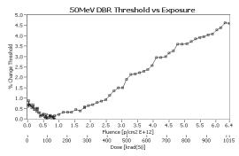
Fig. 15 Change in lasing threshold of JDSU DBR laser measured during 50 MeV proton irradiation.
