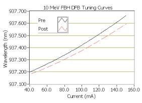
Fig. 2 Tuning curves of the FBH DFB laser before and after 10 MeV proton irradiation.
