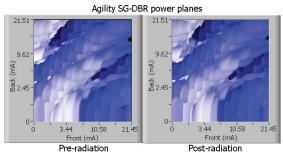
Fig. 9 Power planes scanning Front and Back sections, with Gain/Phase/SOA = 144.9/4.6/100 mA.
