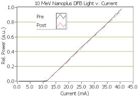
Fig. 3 Nanoplus DFB LIs pre- and post-irradiation.
