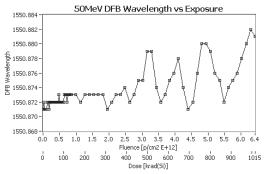
Fig. 14 In-situ measurement of Avanex DFB wavelength during 50 MeV exposure.
