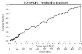
Fig. 13 In-situ change in lasing threshold of Avanex DFB exposed to 50 MeV protons.
