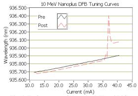
Fig. 4 Tuning curves of Nanoplus DFB at 37 °C.
