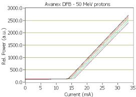
Fig. 12 LIs of Avanex DFB during radiation exposure at fluence =  $0 - 1.8 \times 10^{13}$  cm<sup>-2</sup> in increments of  $3.6 \times 10^{12}$  cm<sup>-2</sup>.
