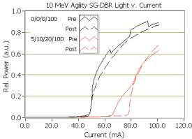
Fig. 11 Pre- and post-irradiation LIs of Agility SG-DBR, ramping Gain with Phase/Front/Back/SOA at two settings, 1) 0/0/0/100 mA and 2) 5/10/20/100 mA.
