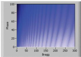
Fig. 8 Example of a measured power plane (Bragg vs. phase) of the JDSU DBR laser measured during proton exposure.
