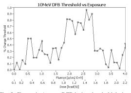
Fig. 5 Change in Avanex DFB lasing threshold during 10 MeV proton exposure
