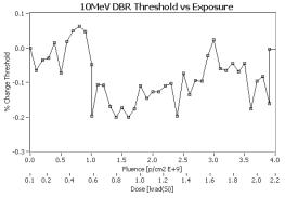
Fig. 7 Measured change in threshold current of JDSU DBR laser during 10 MeV irradiation
