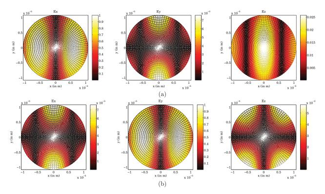
Figure 5. Three components of the electric field  $(E_x, E_y \text{ and } E_z)$  in the case of a two-beam multi-axial combiner. The baseline is along the x-axis and the beams are linearly-polarized along the (a) x-axis and (b) y-axis.
