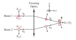
Figure 2. Schematic combination of linearly polarized beams. Depending on the initial orientation of the polarization, the focusing optics introduces a longitudinal component of the electric field.
