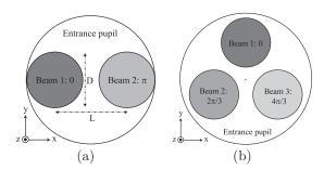
Figure 4. Schematic entrance pupil for the combination of (a) two beams located along the x-axis and (b) three beams. There is a phase-shift between the beams in order to have on-axis destructive interference. The diameter of the beams is D and the distance between the beams in the entrance pupil is L.
