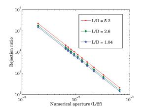
Figure 6. Rejection ratio as a function of the effective numerical aperture L/2f for different values of the ratio L/D.
