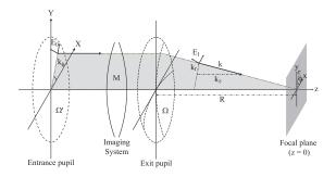
Figure 3. Schematic overview of the studied Light distribution in the entrance configuration. pupil  $E_0(k_r, k_{\phi}, 0)$  is mapped to the exit pupil  $E_1(k_r, k_{\phi}, k_z)$  via an aplanatic imaging system, denoted by the operation M. The field distribution in the focal region is then obtained by integration over the exit pupil. The focal plane is the plane z = 0.
