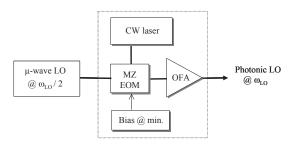
Fig. 3. Photonic LO based on double-sideband modulation with carrier suppression (DSB-CS).
