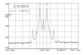
Fig. 6 : Optical spectrum of the 25 GHz photonic LO
