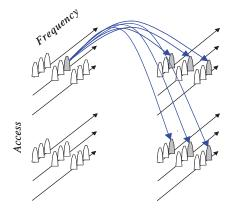
Fig. 2. Channel cross-connection capabilities with access port and frequency sub-band interchange.
