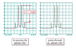
Fig. 11. 2-tone linearity in the microwave photonic crossconnect
