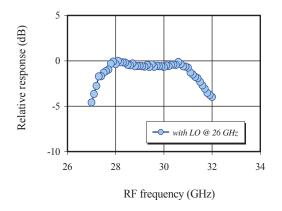
Fig. 8. Photonic RF frequency-conversion : frequency response with LO @ 26 GHz
