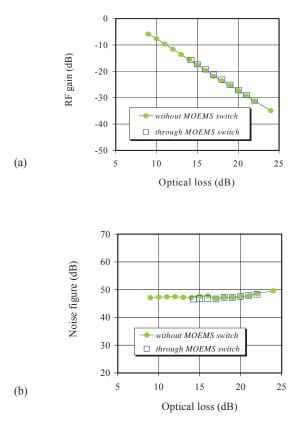
Fig. 10. RF gain (a) and Noise Figure (b) of the microwave photonic cross-connect
