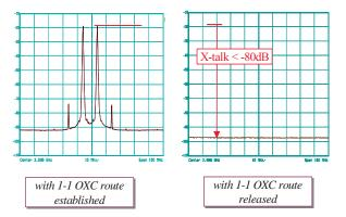
Fig. 12. RF crosstalk in the microwave photonic crossconnect
