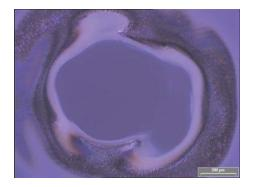
Fig. 2: Deposit on the exit window after a 100°C test with an epoxy based glue
