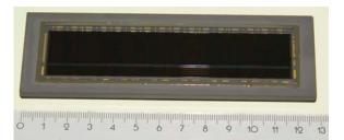
Fig. 7. View of the sensor in PGA package.
