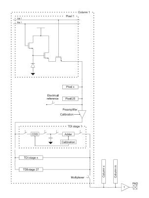
Fig. 4. PAN sensor column architecture
