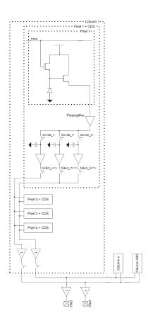
Fig. 6. XS sensor column architecture
