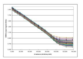
Fig. 12. Preliminary PAN pixel response curves with high preamp gain low adder gain (NTDI=8)
