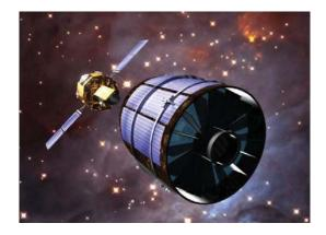
Fig. 5: Artist view of the Detector and Mirror Spacecraft flying in formation at L2.
