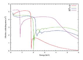
Figure 4: Preliminary estimates of effective area versus photon energy for different X-HPO coatings (without multi-layer coatings).
