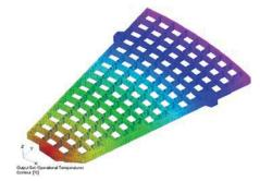
Figure 3: X-HPO petal structure – FEA model (courtesy of *Kayser-Threde*).
