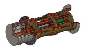
Fig. 1: Adiabatic Demagnetization Refrigerator under development for XEUS (courtesy of *MSSL*).
