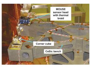
Fig. 12 : Sensor installation on the HSOB
