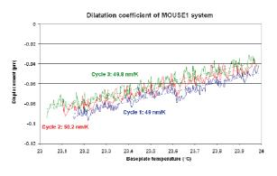
Fig. 11 : Displacement measurements
