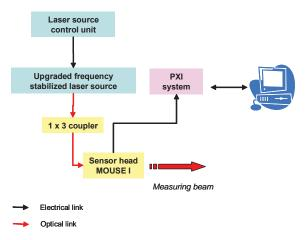
Fig. 3 : Architecture of the setup
