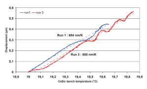
Fig. 13 : Repeatability of CeSiC expansion measurements
