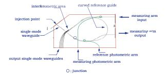
Fig. 1: Layout of the optical circuit
