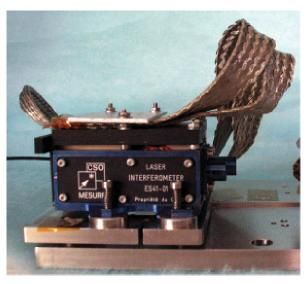
Fig. 9 : MOUSE with thermal braid
