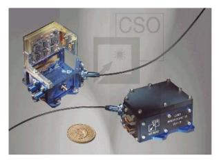
Fig. 2 : MOUSE I sensor head
