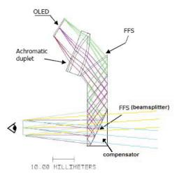
Fig.5. Schematic layout of the optical system
