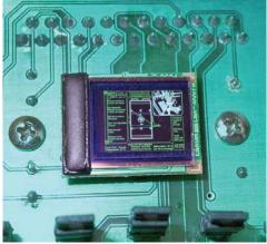
Fig.6. Photography of the SVGA+ OLED microdisplay.
