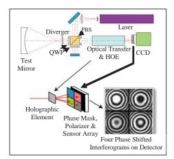
Fig. 1. Simultaneous phase-shifting interferometer (PhaseCam).
