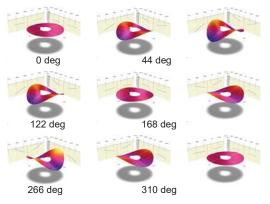
Fig. 8. Measurement of vibration of a disk (408 Hz.).
