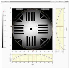
Figure 13. Surface change obtained from measurement of a 1m carbon fiber target.
