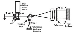
Figure 6. Simultaneous phase-shifting Fizeau – short coherence length source.
