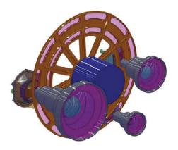
**Fig. 1** : OCAPI instrument concept. There are three wide field-of-view optics sharing the same filter wheel. SWIR optics is the largest one, and UV the smallest
