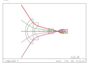
Fig. 5 : Optical design for the visible channels set
