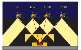
Fig. 2 : Principle of directional signature measurement. As the satellite goes along its orbital path, a surface target is within the instrument FOV for about 5 mn. During that time, the radiometer makes about 15 acquisitions and the target reflectance is measured under different geometries.
