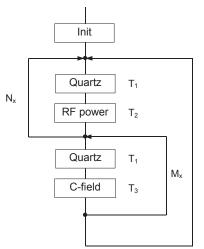
Fig. 7: Software architecture of the OSCAR lock loops.
