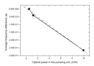
Fig. 6: Relative frequency difference of OSCAR and an active hydrogen maser for different optical pumping powers. The slope of the linear fit is  $-2.7 \times 10^{-12} \text{ mW}^{-1}$ .
