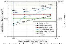
Fig. 4: Noise budget and overall SNR of OSCAR.
