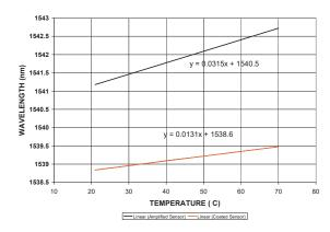
Fig. 7: Measured temperature response of bare FBG (red curve) and packaged FBG with MEMS-amplified thermal sensitivity (dark curve).
