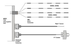
Fig. 3: Schematic of FSD fiber-optic sensor signal harness.
