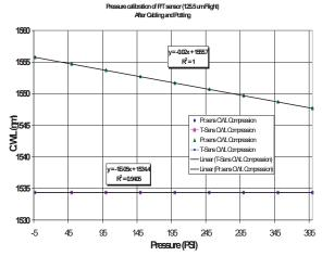
Fig. 5: Response of the P/T pressure-sensing and temperature sensing FBGs to the applied pressure.
