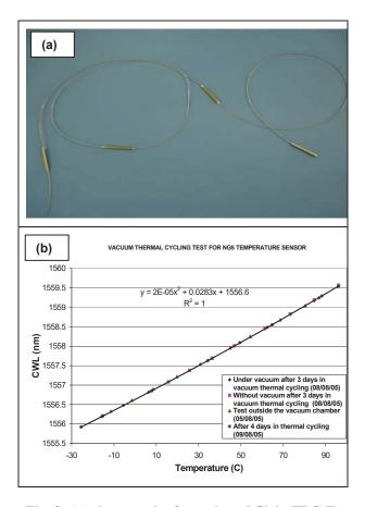
Fig. 8: (a) photograph of a packaged flight FBG T-sensor line with protective cabling and four sensors, (b) test results for one of the FSD FBG T-sensors.
