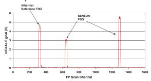
Fig. 9. Measured spectrum of fiber-optic line containing one internal athermal reference FBG and two external FBG sensors, as obtained using the FSD interrogation unit.
