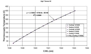
Fig. 6: High-T sensor calibration after repeated thermal cycling.
