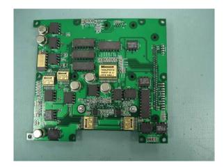
Fig. 3: Photograph of the low-power flight DAQ (Data Acquisition) PCB.
