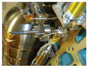
Fig. 4: Photograph of flight P/T sensor integrated with the SSTL propulsion system for Proba-2.
