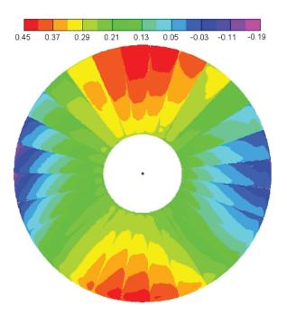
Fig. 5 The field of the normal displacements (related to best-fit paraboloid, Load Set 2).
