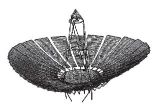
Fig. 3 The view of the deformed model for Load Set 2.
