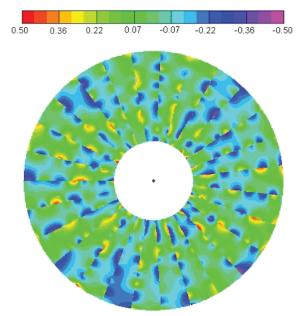
Fig. 7 The field of the normal displacements (the manufacturing and installation faults and the space influence).
