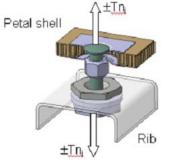
Fig. 6 The join points shell/frame and the enforced motion.
