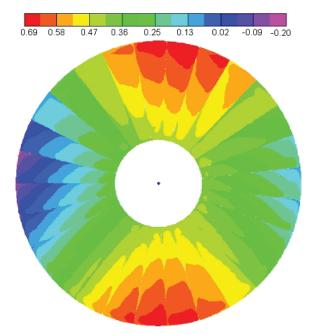
Fig. 4 The field of the normal displacements (in mm, the rigid-body motions of reflector are excluded, Load Set 2)
