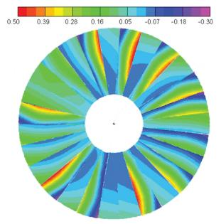
Fig. 9 The field of the normal displacements (the space influence on composite pipes).
