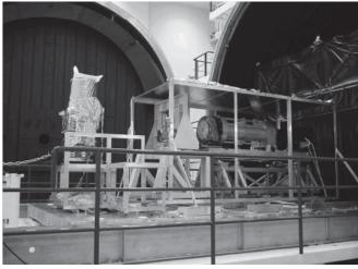
Fig. 1. LUCE FM (left) in the 6m space chamber
