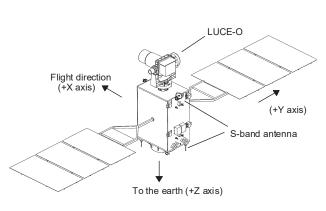
Fig. 3. In-orbit satellite configuration of OICETS
