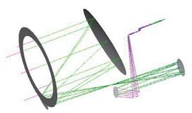
Figure 3. Asymmetric Korsch all reflective three mirror design at WFE  $<\lambda/20$  and suitable pupil plane locations capable for in-field guiding by  $+-1^{\circ}$
