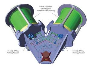
Figure 1. Single test mass payload configuration for LISA. The inertial sensor is located on a single optical bench and similar to the LISA Pathfinder
