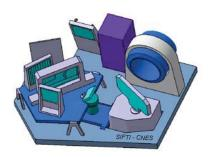
Figure 10: SIFTI opto-mechanical layout
