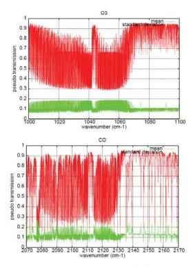
Figure 6: Average (red) and standard deviation (green) of atmospheric transmission for  $O_3$  (above) and CO (below) region, among 232 atmosphere cases.
