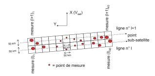
Figure 1: schematic of the agile pointing along two successive swaths
