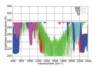
Figure 2: contribution of selected molecules in the atmospheric spectrum : H<sub>2</sub>0 (green), CO<sub>2</sub> (blue), O<sub>3</sub> (pink), CO (cyan). 4AOP simulations.
