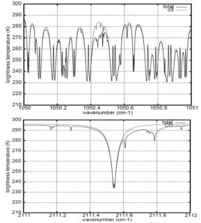
Figure 3: brightness temperature (K) as a function of wavenumber for a narrow spectral band (1 cm<sup>-1</sup>): at SIFTI spectral resolution, the O<sub>3</sub> absorption lines are not resolved (top) but the CO absorption lines are resolved (bottom).
