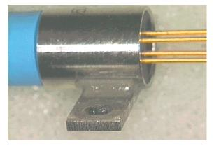
Fig. 8. Epoxy fixing the receiver metal parts.
