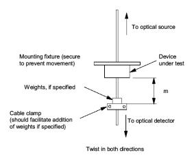
Fig. 11. Set schematic for cable retention test.(fibre cable assembly)
