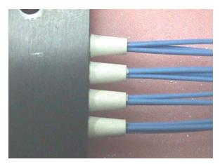
Fig. 10. Splitters output of the fibres
