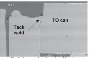
Fig. 5. Cross section of a tack weld crack.
