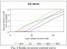
Discussion with the manufacturer led to the conclusion that at low temperatures a second laser mode starts oscillating and only one mode is coupled into the fibre pigtail leading to the kink in the power-current curve.
