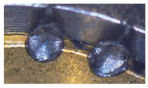
Fig. 4. Cracks in the tack welds
