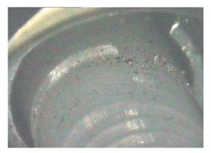
Fig. 9. Internal aspect of the connectors after matedemate test.
