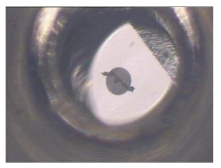
Fig. 15 Particle found on the end of the fibre after opening the receiver.
