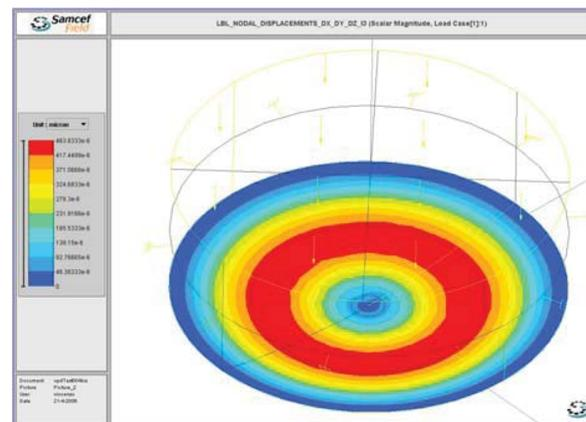
Fig. 6. Sag correction for an odd aspheric surface.
