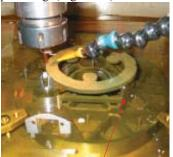
Filtering blades finished by EDM
