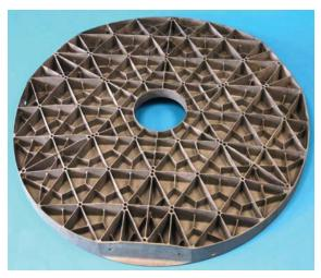
Figure 15 View of the mirror after infiltration
