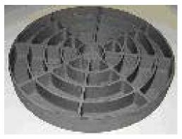
Figure 13 View of rear face mirror with Sic CVD coating
