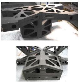
Fig. 13. View of HSOB greenbody once assembled
