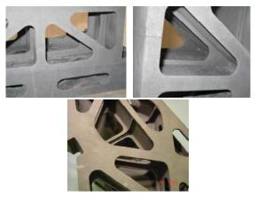
Fig. 10. HSOB inner cells due to ribs & skins
