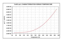
Fig. 2. CeSiC CTE is quasi-null at cryogenic T°
