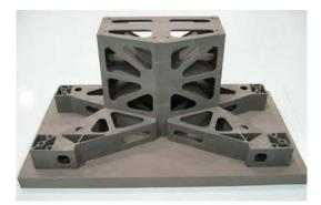
Fig. 15. HSOB after sand blasting
