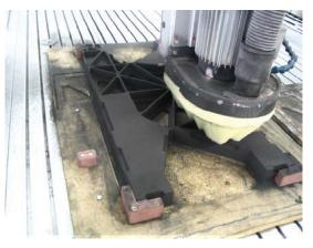
Fig. 9. HSOB plate-form greenbody during milling
