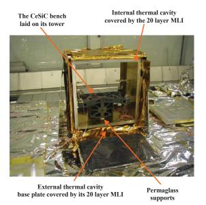
Fig. 20. HSOB test configuration cavities opened
