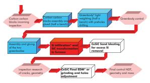
Fig. 7. CeSiC manufacturing simplified scheme
