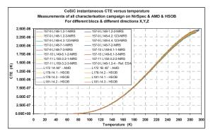
Fig. 26. CeSiC CTE homogeneity measured
