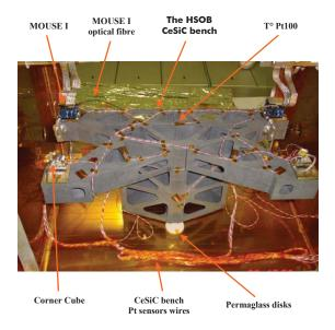
Fig. 21. HSOB zoom on the equipped bench
