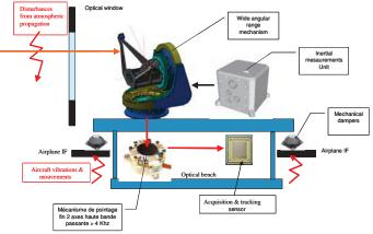
Fig.8: Pointing, Acquisition & tracking architecture
