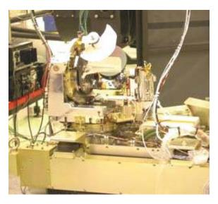
Fig.5: LOLA optical terminal during modal survey
