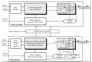
Fig.10: Laser communication unit
