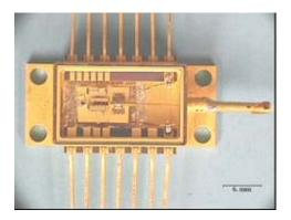
Fig.9: LOLA European 0.8µm laser diode
