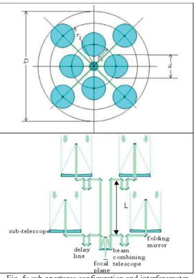
Fig. 5: sub-apertures configuration and interferometer optical concept
