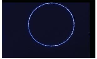
Figure 10. This shows an image of the Fabry Perot fringes. The filter bandwidth is 32 pm with a peak transmission of 55 %.
