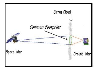
Figure 3: Schematic diagram of the different beam divergences between the space and ground based lidars. The so called common footprint is shown.
