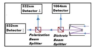
Figure 1: Block diagram for the lidar receiver.
