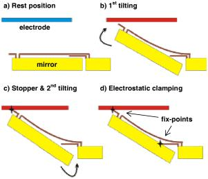
Fig. 1: Schematic view of the actuation of the mirror and electrostatic locking mechanism
