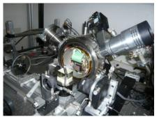
Fig. 3: Cryogenic set-up mounted on the interferometric bench.
