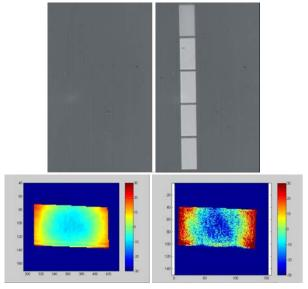
Fig. 4: Testing of a micro-mirror array at 92K (0V and 90V applied); 100x200 μm<sup>2</sup> mirrors surface deformation at room temperature and at 92K
