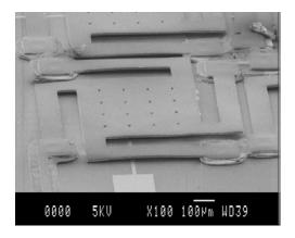
Fig. 5: View of a polymer actuator with a 580µm plate by scanning electron microscope
