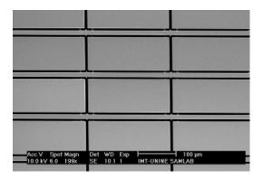
Fig. 2: SEM image of a small 5x5 micro-mirror array
