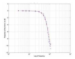
Fig. 6: Frequency response of the polymer-based actuator. A theoretical curve of a second-order system with  $f_r$ =6.5kHz and Q=0.7 is fitted
