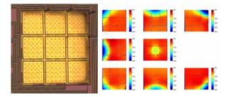
Fig. 7: a) Micro-deformable mirror prototype with 3x3 actuators ( $200x200\mu m^2$  for each actuator) and a continuous membrane on top. Structural material is polysilicon; b) Influence functions of LAM prototype (one actuator, middle right, is stuck on the substrate)
