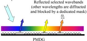
Fig. 10: Principle of wavelengths selection by using a PMDG. Selected wavelengths are reflected while others are diffracted and blocked by a mask in Fourier plane.
