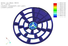
Fig. 11 Thermal stress on the wheel
