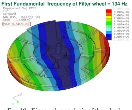
Fig. 10 Eigen value analysis of the wheel
