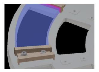
Fig. 12 Section of wheel showing buttons
