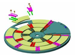
Fig.2. Filter wheel assembly
