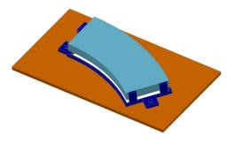
Fig. 7 Flexure Mount
