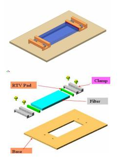
Fig.5 Assembly and Exploded Views of Soft Mount
