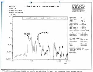
Fig. 13 Wheel modes in dynamic tests
