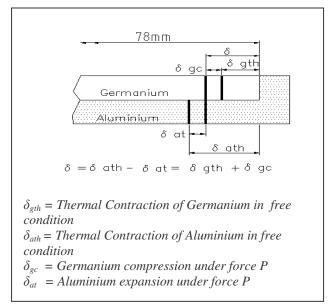
Fig. 3 Behaviour under bimetallic force
