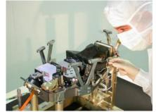
Fig. 4: SiC focal plane prior to integration
