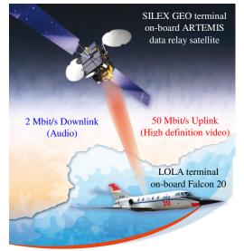
Fig. 1: The LOLA bi-directional optical data link between an aircraft and the Artemis GEO Relay satellite
