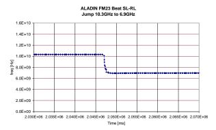
Fig. 9. 3.4 GHz jumping verification of SL-RL beat signal.
