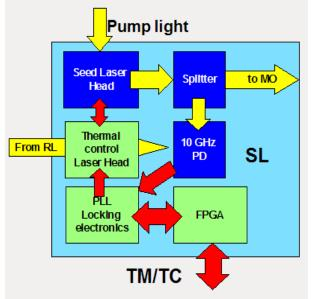
Fig. 3. SL design: Optical fiber connections are shown in yellow, electrical signals in red. TM/TC denotes telemetry and telecommand flows.
