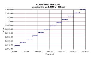
Fig. 8. Frequency stepping verification "fine up". Only a small portion of the duration of the experiment is shown.
