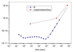
Fig. 6. Allan variance (in Hz/Hz) of the RL cavity (blue) compared with the AEOLUS mission requirements (red).
