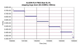
Fig. 7: Frequency stepping verification "large down". Only a small portion of the duration of the experiment is shown.
