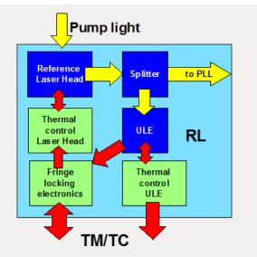
Fig. 2. RL design. Optical fiber connections are shown in yellow, electrical signals in red. TM/TC denotes telemetry and telecommand flows.
