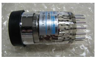
Fig. 7. PHEBUS NUV photomultiplier
