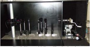
Fig. 8. Photomultiplier calibration bench
