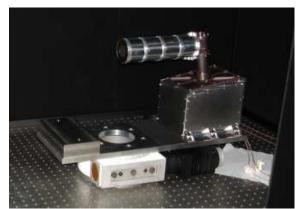
Fig. 5. Baffle optical test bench
