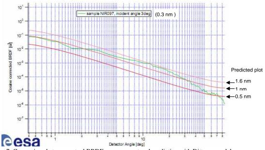
Figure 7: Comparison between actual BRDF measurement and prediction with Dittman model
