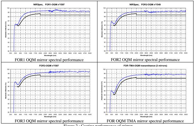
Figure 2 : Coating performance of mirror
