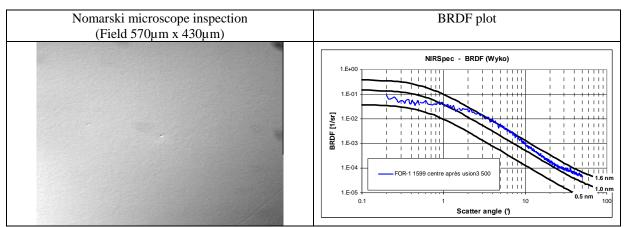
Figure 6: Process performance for Flight Model mirror (µ-roughness 0.4 nm)
