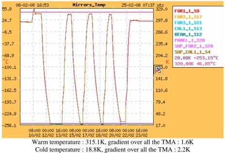
Figure 5 : Thermal cycling of FOR OQM TMA cryo test
