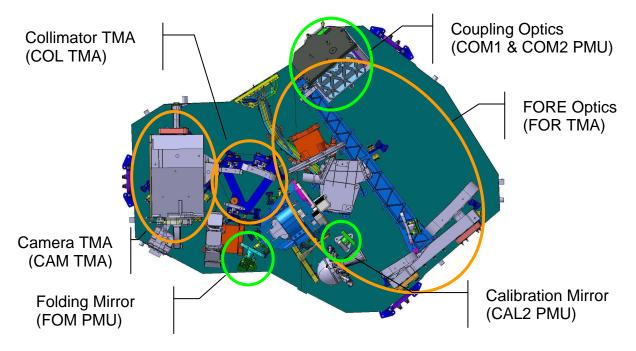
Figure 1 : Top view of the NIRSpec instrument with Sagem contribution
